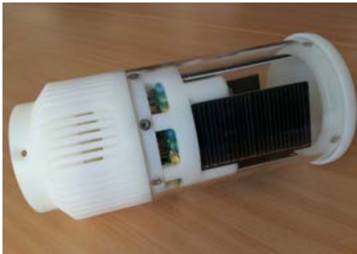
Figure 5.4. Electric devices to be mounted on posts which emit variable sounds and flashes of light.
