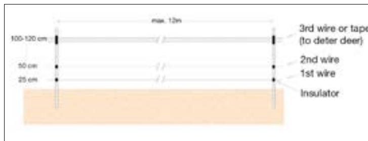
Figure 3.1. Diagram of an electric fence suitable for wild boar and roe deer.
