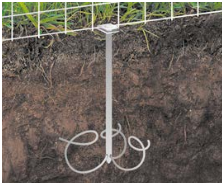
Figure 2.5. Peg for anchoring the mesh to the ground.
