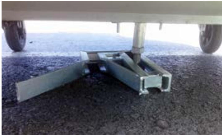
Figure 9.4. System for attaching the container to the anti-tipping platform.
