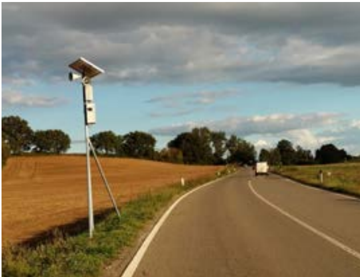
Figure 5.2. Devices activated by the detection of target species that emit recorded sounds (which vary depending on the species).
